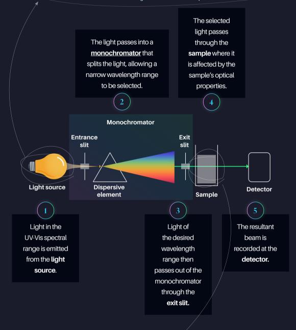
It is important to choose the right instrument and cuvette type for your sample. For example, most plastic cuvettes are not suitable for UV absorption studies as they absorb UV light.
