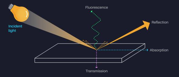
Typically, in UV-Vis spectroscopy, **absorbance** is measured.
