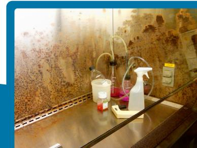
Stainless-steel interior quickly erodes when coated with bleach or other corrosive disinfectants.
